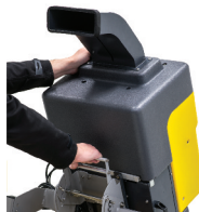
The X-PAD head can be tilted to dispense at the point where paper void fill is needed
